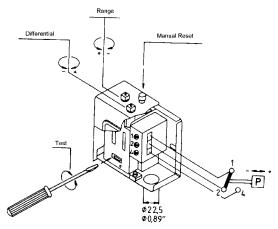
**NOTE:** The cut-in (start point) presssure is the cut-out (range adjusting setting) pressure minus the differential setting.
