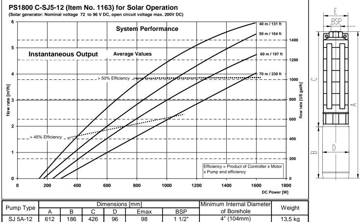
An irradiation value and the required head in meters are given for a certain solar pumping system.
