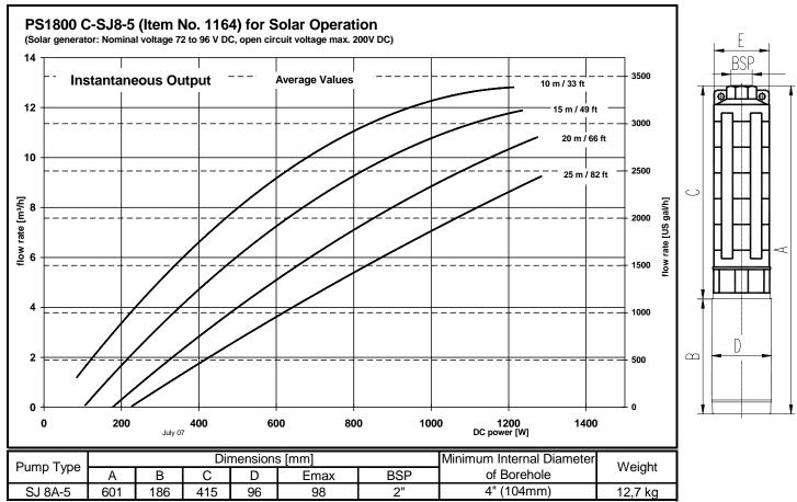
An irradiation value and the required head in meters are given for a certain solar pumping system.
