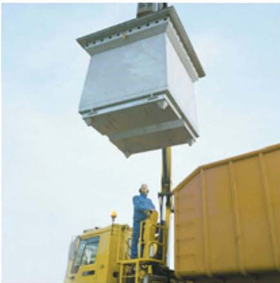
Lifting, emptying and locking are controlled via a central, integrated mechanism
