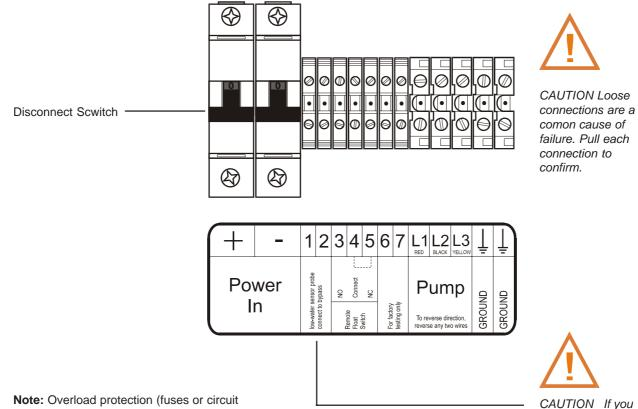
**Note:** Overload protection (fuses or circuit breaker) is NOT required in the solar array circuit.
