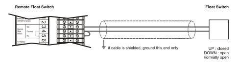
Wiring a "normally closed/reverse action switch" Connect the switch to termins 4 and 5. Closing (connecting) the switch turns the pump ON
